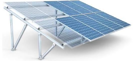
**H2100–116** is an aluminum structure solution for 3 panels portrait or 4 panels landscape. The system is provided with all needed clamps, connection base plates (to concrete blocks or steel piles) and stainless steel assembly screws in preassembled package. The inclination is 20 –30 / or can be customized as per exact requirements for large scale projects.
