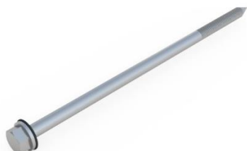
DIN7504-K SELF DRILLING SCREW 6,3x150 (EX-7626615000) or 6,3x110 (EX-7626611000) GALVAN+EPDM
