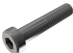
ALLEN BOLT DIN912/ISO4762 M8xLENGTH INOX A2* *Length of allen bolt depends on the thickness of the PV panel
