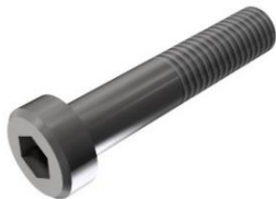
ALLEN BOLT DIN912/ISO4762 M8xLENGTH INOX A2* *Length of allen bolt depends on the thickness of the PV panel
