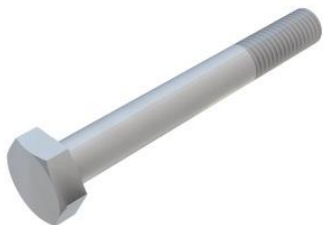
HEXAGON BOLT ISO4017 M10x80 A2 INOX (EX-7622108001)
